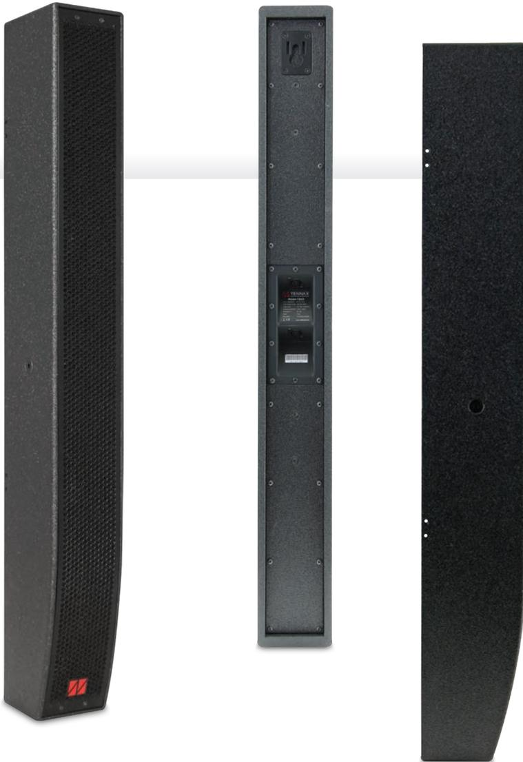
The name axon comes from Latin and is translated as line or wave. Both apply equally to this loudspeaker: the close arrangement of the 12 x 3" wideband loudspeakers in a vertical line achieves particularly good coupling, thus creating a flat wavefront over a wide frequency range.
